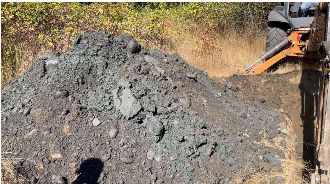
Top left – top disturbed layers (top 7 ft) with approximately 50% gravel or larger. Top right – material below 7 ft depth comprised of silty sand with approximately 30% gravel or larger. Bottom – spoils pile showing mainly the gray gravelly silt from 2 to 7 ft depth.
