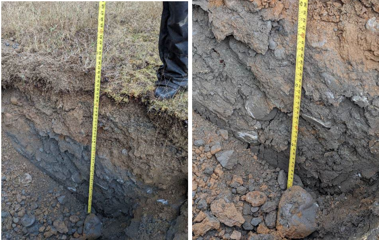
Top - Brown sandy loam above grey sandy loam with gravels and small cobbles; Bottom - close up of grey silty sand with approximately 30% cobbles
