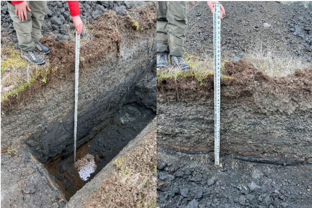
Left – Clear soil horizons; Brown silty soil above gray sand above gray clay.
