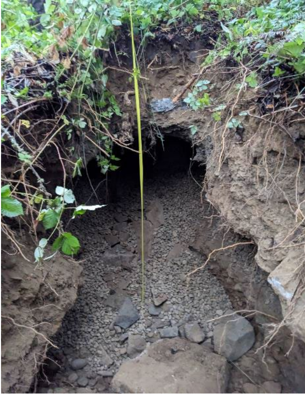
Top - pit taken in berm, 4 to 5-foot boulders in berm; Bottom - start of natural gravels at 12 feet, caving in before 15 foot target
