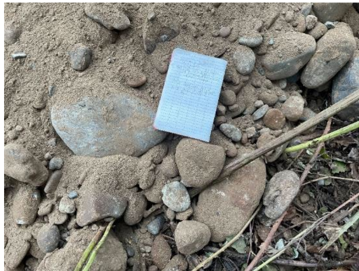
Top – coarse layer at 6 foot depth; Bottom – Close-up of coarse alluvial layer
