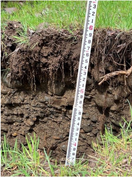
Right – Close up of poorly sorted gravel in a fine/sandy matrix.
