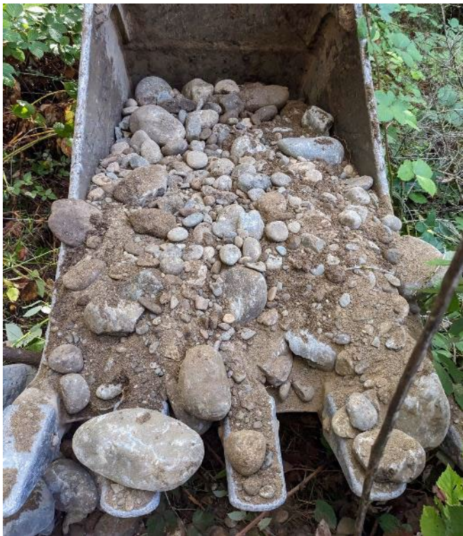
Top - Pit taken in berm, gravels and cobbles at surface, larger cobbles at 6-7 feet; Bottom - close up of cobbles and gravels from bottom of pit
