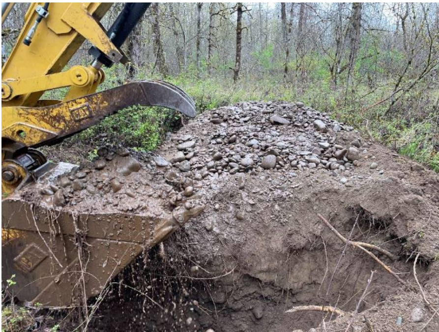
Top – Gravel and cobbles in a fine matrix, groundwater at
