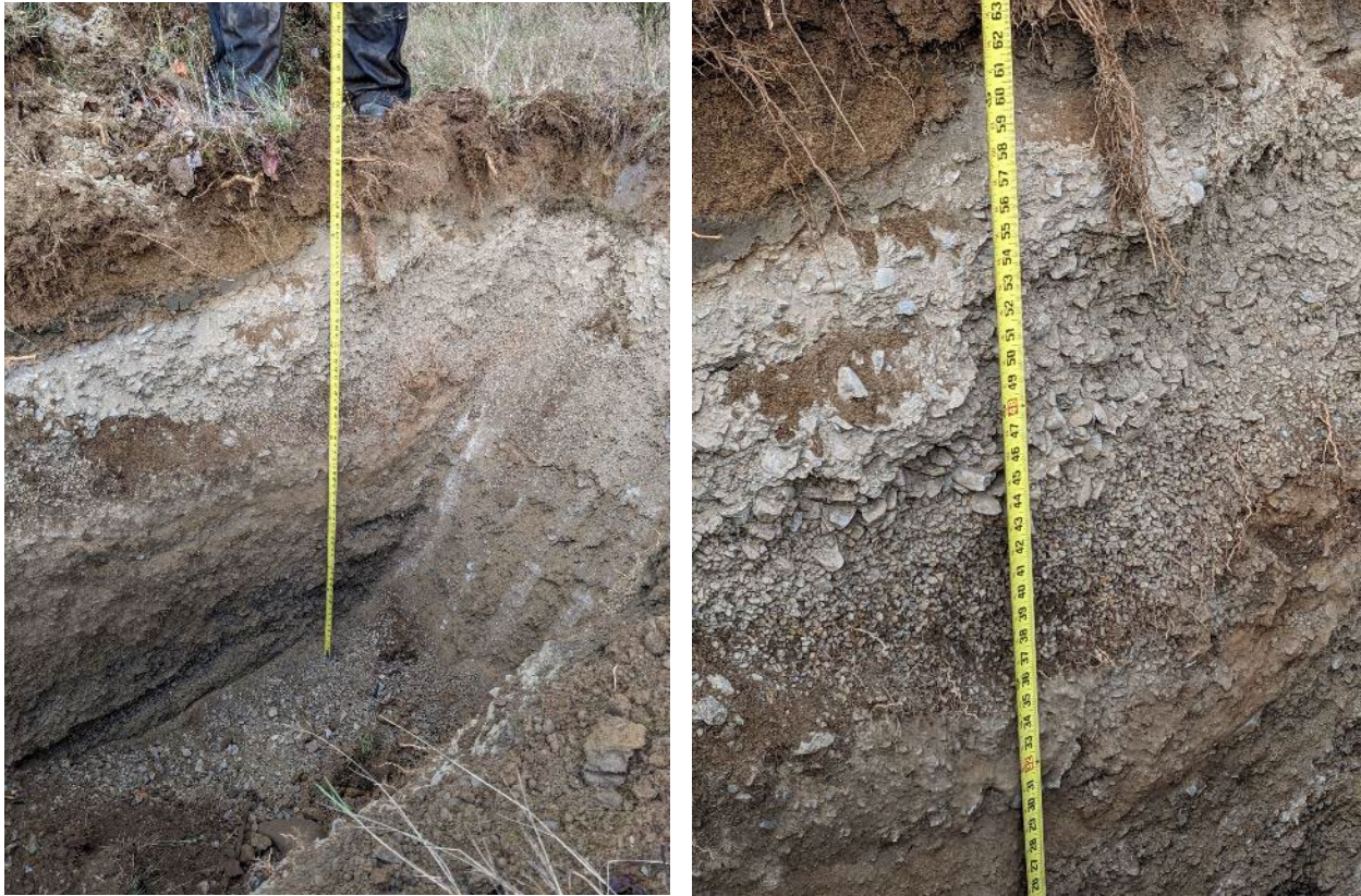
Left - Silty loam with crushed rock and pea gravel throughout pit; Right - close up of crushed rock layer at 1.25 feet
