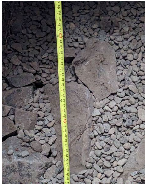
Top - pit taken in berm, 4 to 5-foot boulders in berm; Bottom - start of natural gravels at 12 feet, caving in before 15 foot target
