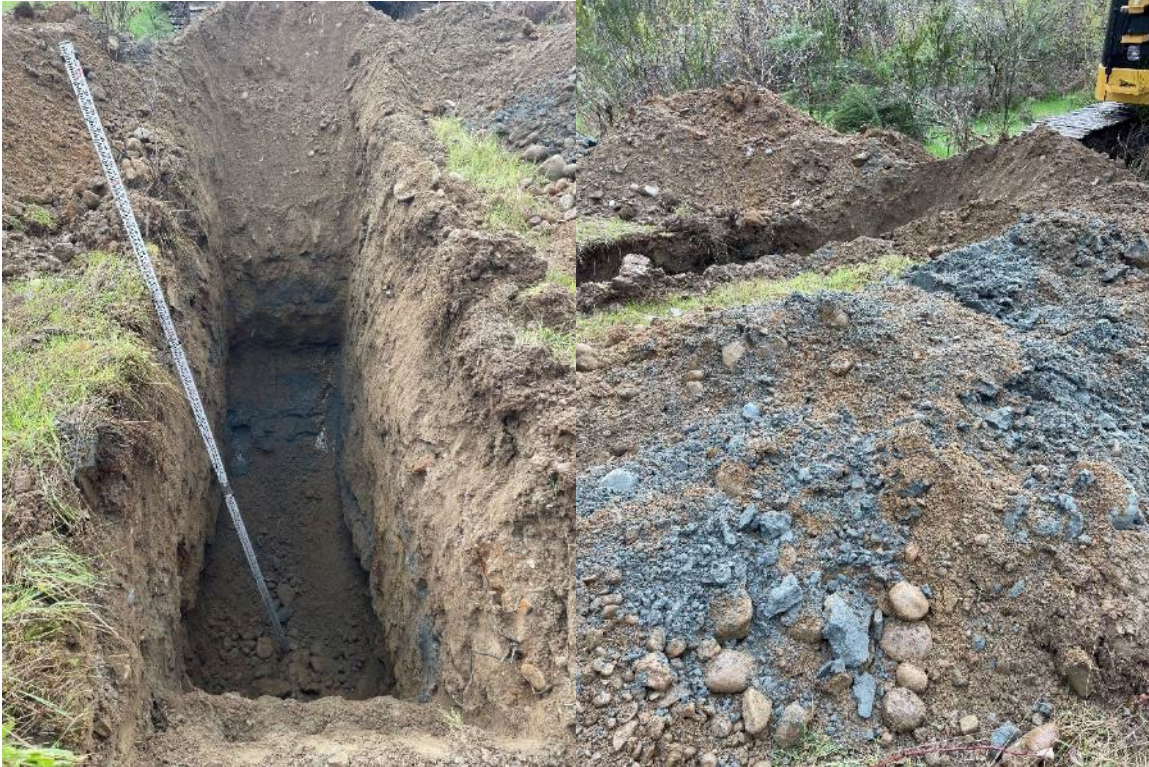
Left – Sand, silt, and cobbles interbedded with gray clay.
