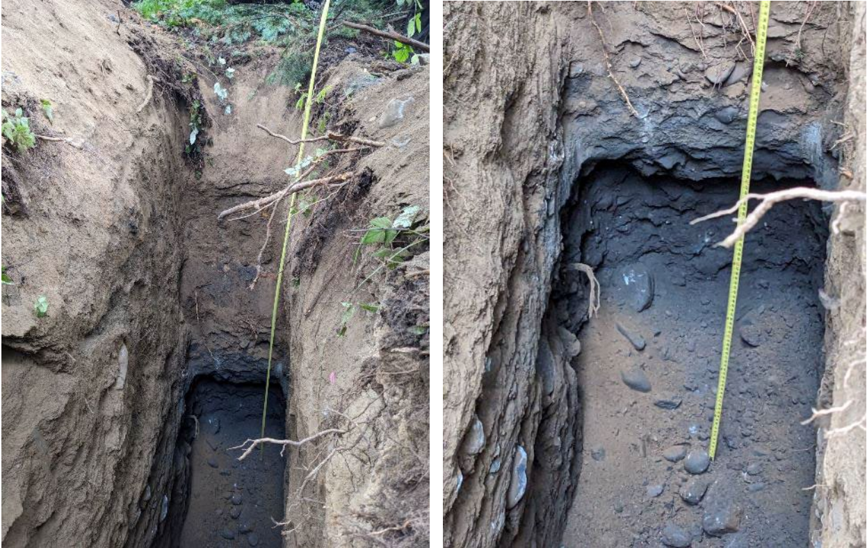
Left - Brown silty sand with occasional 10-12 inch cobbles; Right -close up of dark grey material starting at 9 feet, with 10-12 inch cobbles
