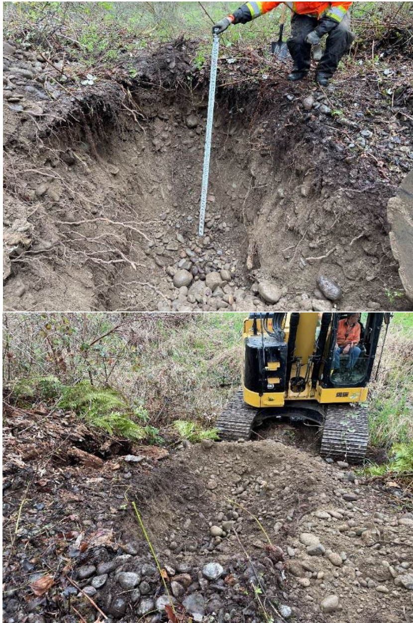
Left – Gravel and cobbles in an unconsolidated matrix of fines.
