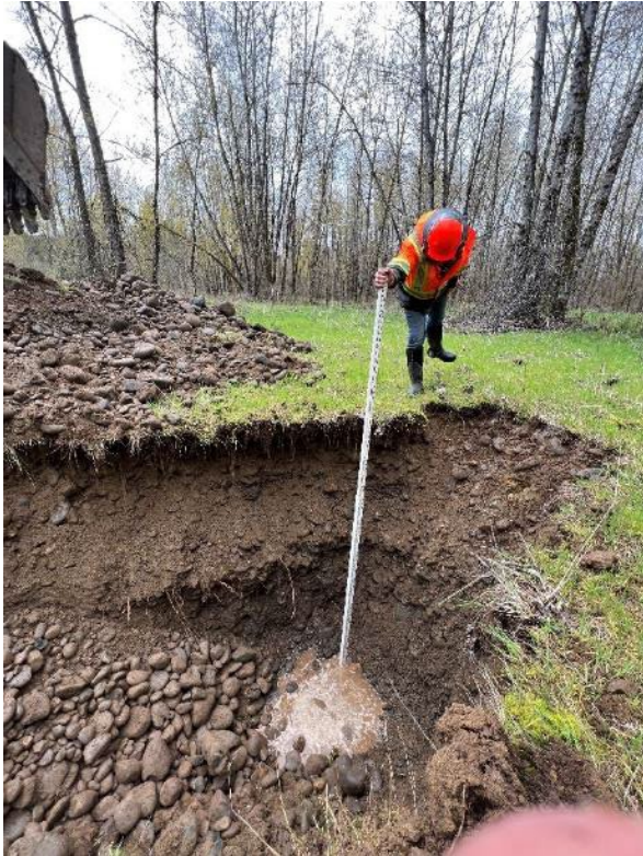
Left - Unconsolidated soils mixed with rounded gravel and cobbles
