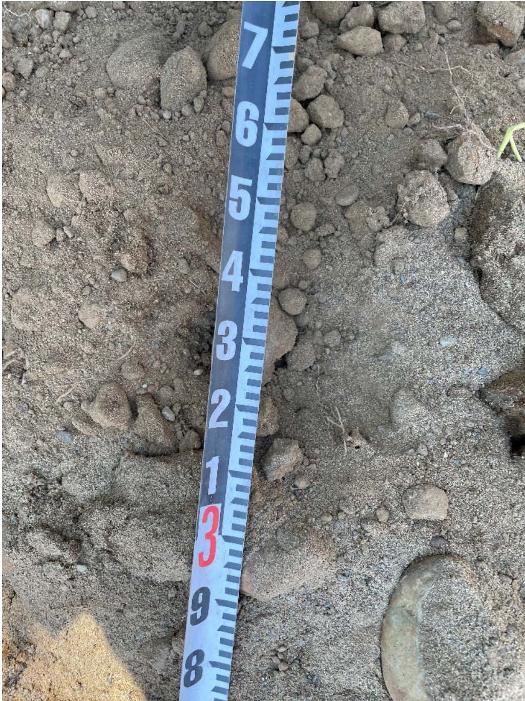
Top 3 feet of Test Pit 7 (sand with approximately 20% gravel or larger)
