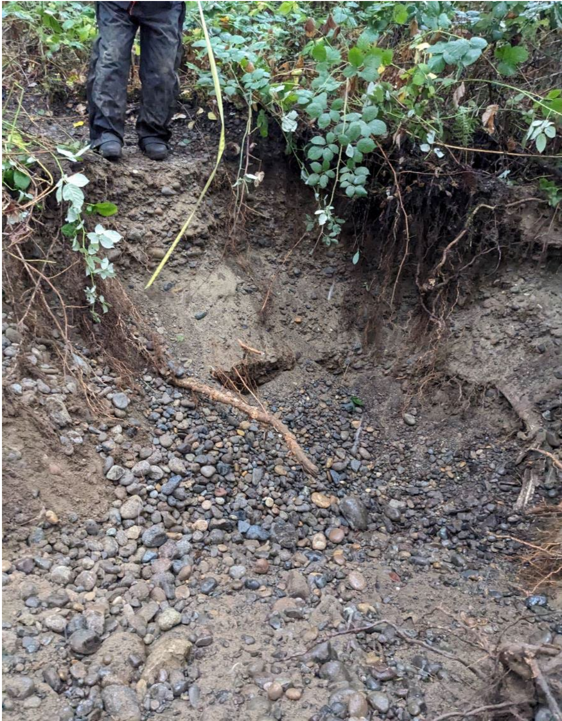
Above - Close up of gravels and cobbles in bottom of pit
