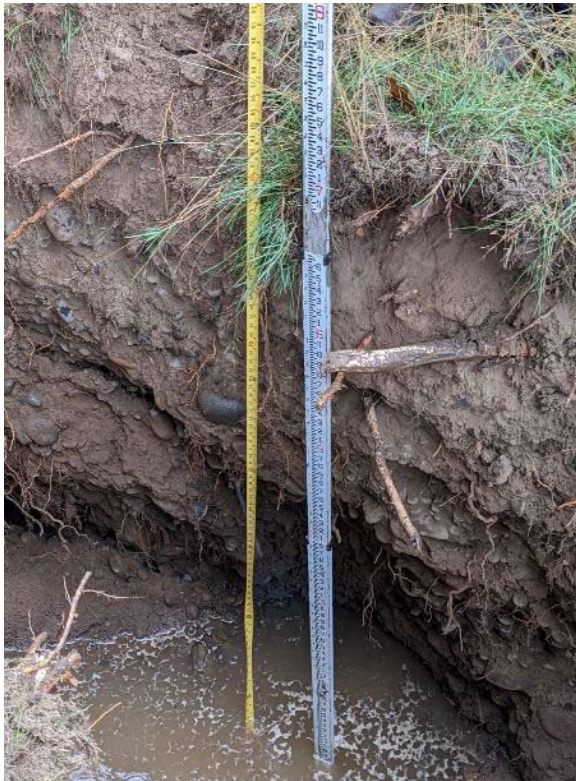
Top - test pit with water table at 73 inches; Bottom left - top with thick roots, cobbles and gravels start at 7 inches; Bottom right - >50% coarse materials
