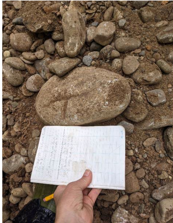
Left - Pit in berm, dark brown loam with roots and plant material in top of pit, silty sand with 60% cobbles at 10 inches; Right - close up of well sorted material at bottom of pit
