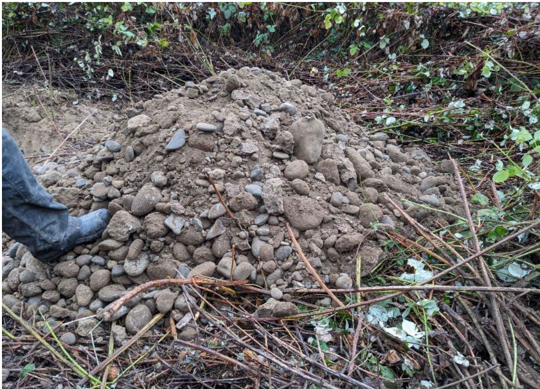
Top left - thick tree roots at surface; Top right - Cobbles and gravels at 7 feet; Bottom - larger cobbles with conglomerate material at bottom of test pit
