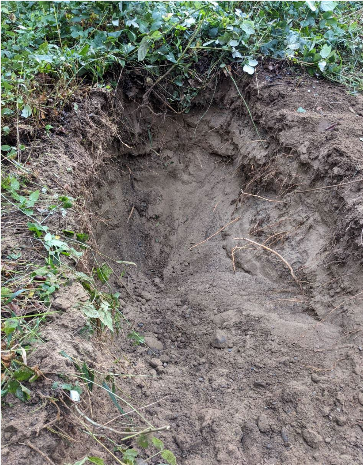
Above - Brown sand with a few cobbles at bottom of pit
