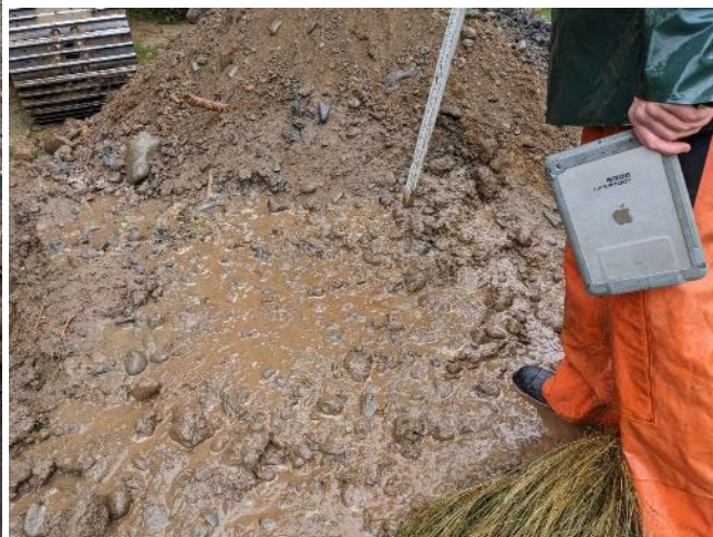
Top - test pit with water table at 73 inches; Bottom left - top with thick roots, cobbles and gravels start at 7 inches; Bottom right - >50% coarse materials
