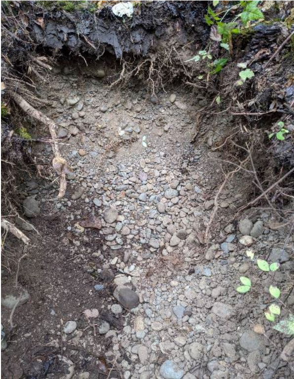
Left - Pit in berm, dark brown loam with roots and plant material in top of pit, silty sand with 60% cobbles at 10 inches; Right - close up of well sorted material at bottom of pit
