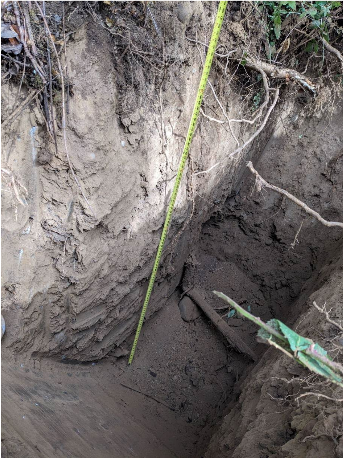
Above - Pit taken in berm, silty loam for majority of pit, bottom of pit with woody debris and soils with redox
