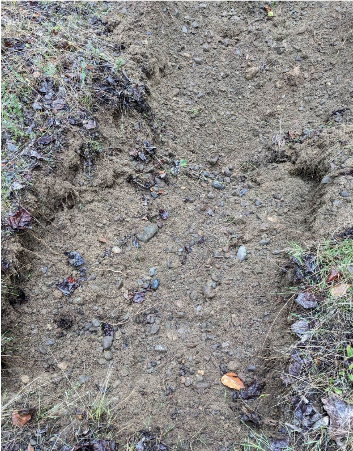
Above - Pit with brown sand with gravels and cobbles to 4 inches
