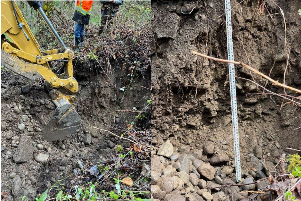
Left – Large chunks of concrete and cobbles in disturbed layer.
